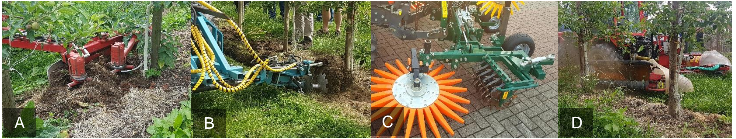
Different types of mechanical weeding devices: Picture A. LADURNER Gyroscopic Crumbler, Picture B. SPEDO disc plough, Picture C. Roll- and fingerhoe combination (Adelhelm & K.U.L.T. Kress), Picture D. LADURNER Thread mower. Photos: N. Oeser, 2018.
